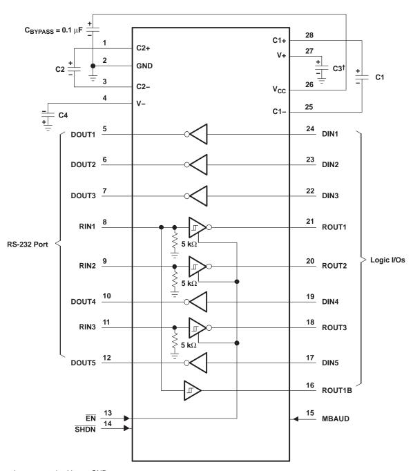
$<sup>^{\</sup>dagger}$  C3 can be connected to  $V_{\mbox{\footnotesize CC}}$  or GND.
