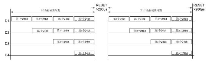
Note: The data of D1 is send by MCU, and D2, D3, D4 through pixel internal reshaping amplification to transmit.
