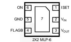
Figure 4. Pin Assignment (Top Through View)
