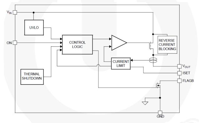
Figure 3. Block Diagram
