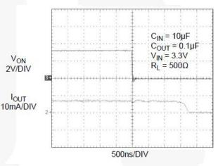
Figure 13. td<sub>on</sub> Response
