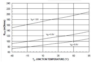
Figure 9. Ron vs. V<sub>IN</sub>
