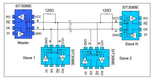
Figure 9 Bus type RS485 half duplex communication network
