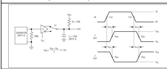
Figure 4 Drive propagation delay
