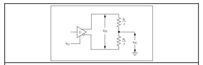
Figure 2 Driver DC test load
