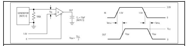
Figure 7 Receiver propagation delay test circuit
