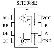
Figure 1 SIT3088E Pin Configuration
