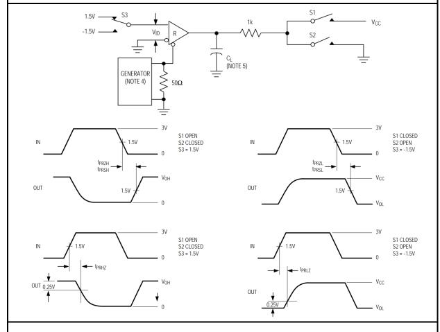
Figure 8 Receiver enable and disable time
