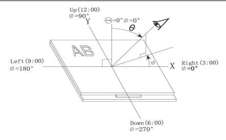
Note 4: Definition of contrast ratio.( Test LCD using DMS501)
