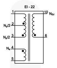
Figure 30. Transformer Specification
