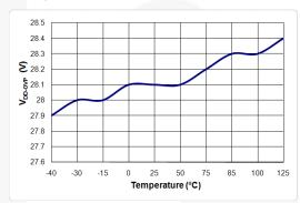
Figure 7. V<sub>DD-OVP</sub> vs. Temperature
