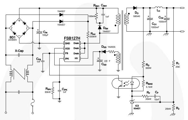
Figure 29. Schematic of Typical Application Circuit
