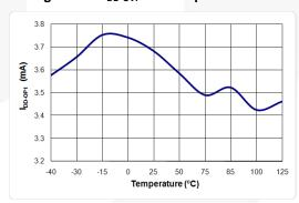
Figure 9. IDD-OP1 vs. Temperature
