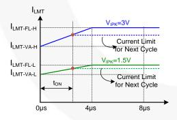
Figure 22. I<sub>LMT</sub> vs. PWM Turn-On Time
