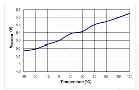
Figure 12. V<sub>FB-OPEN</sub> vs. Temperature
