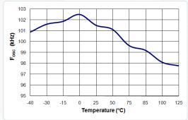
Figure 16. fosc vs. Temperature
