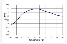
Figure 15. IPK vs. Temperature
