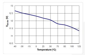
Figure 4. V<sub>DD-ON</sub> vs. Temperature
