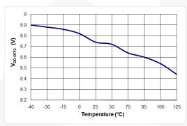
Figure 6. V<sub>DD-OFF2</sub> vs. Temperature
