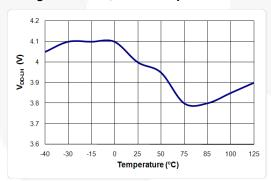
Figure 8. V<sub>DD-LH</sub> vs. Temperature
