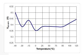
Figure 5. V<sub>DD-OFF1</sub> vs. Temperature
