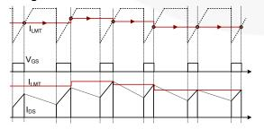
Figure 23. Current Limit Variation with Duty Cycle
