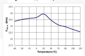
Figure 17. fosc-g vs. Temperature
