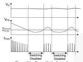
Figure 26. Burst-Mode Operation
