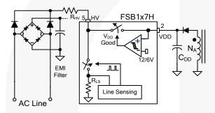
Figure 18. Startup Circuit
