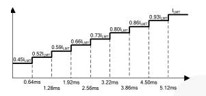
Figure 21. Current Limit Variation During Soft-Start
