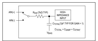
Figure 1. Unbuffered Analog Input Structure
