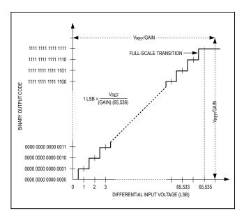
Figure 4. MAX1415/MAX1416 Unipolar Transfer Function
