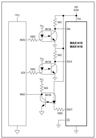
Figure 13. Optically Isolated Interface
