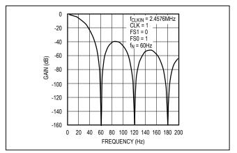
Figure 6. Frequency Response of the SINC<sup>3</sup> Filter (Notch at 60Hz)
