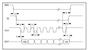
Figure 9. Read Timing Diagram
