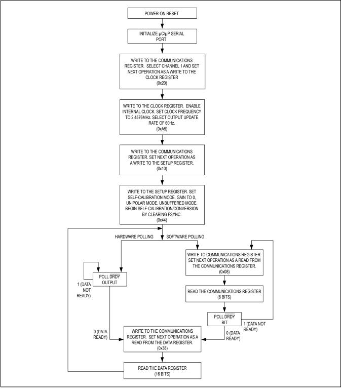
Figure 11. Sample Flow Diagram for Data Conversion
