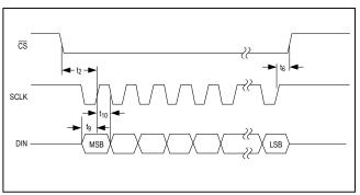
Figure 8. Write Timing Diagram
