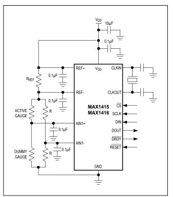
Figure 12. Strain Gauge Measurement
