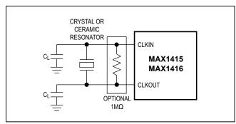
Figure 7. Using a Crystal or Ceramic Oscillator
