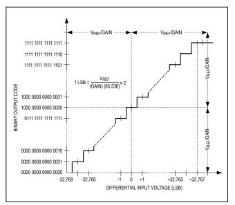
Figure 5. MAX1415/MAX1416 Bipolar Transfer Function
