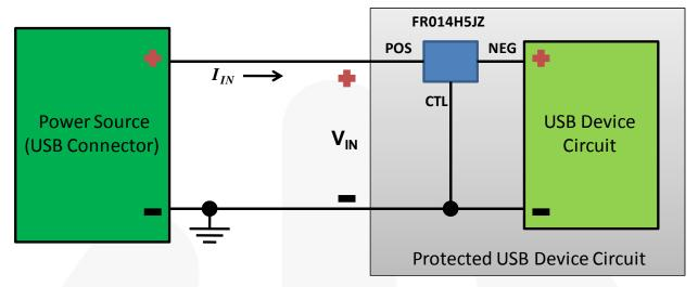
Figure 13. Typical Application Circuit for USB Applications
