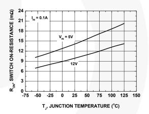
Figure 8. Effective Switch Resistance  $R_{SW}$  vs. Input Voltage  $V_{IN}$
