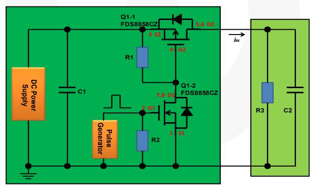
Figure 16. Startup Test Circuit – without FR014H5JZ
