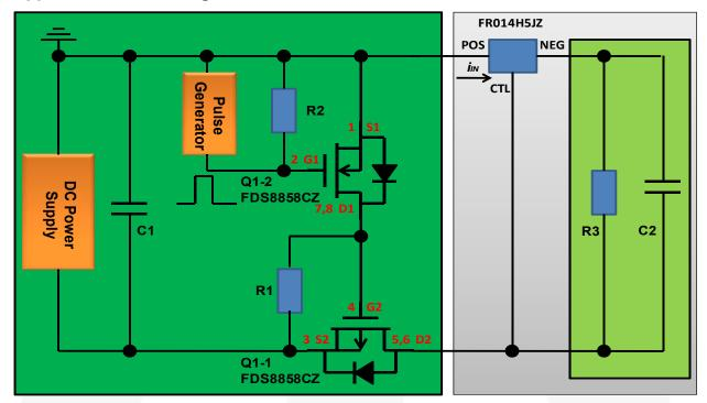
Figure 15. Startup Test Circuit - Reverse Bias with FR014H5JZ
