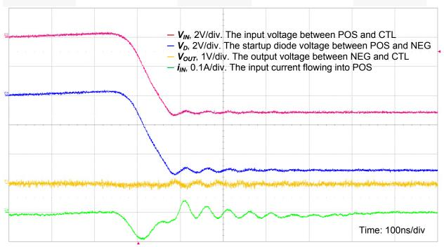
Figure 18. Reverse Bias Startup Waveform, DC Power Source=5V, C<sub>1</sub>=100μF, C<sub>2</sub>=10μF, R<sub>1</sub>=R<sub>2</sub>=10kΩ, R<sub>3</sub>=27Ω
