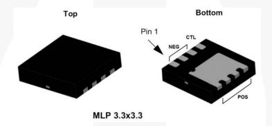
Figure 3. Pin Assignments
