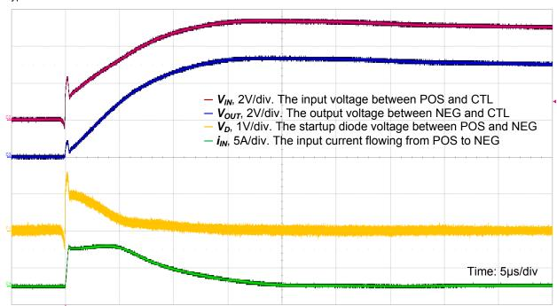
Figure 17. Normal Bias Startup Waveform, DC Power Source=5V, C<sub>1</sub>=100μF, C<sub>2</sub>=10μF, R<sub>1</sub>=R<sub>2</sub>=10kΩ, R<sub>3</sub>=27Ω
