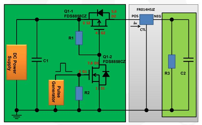
Figure 14. Startup Test Circuit - Normal Bias with FR014H5JZ
