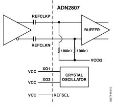
Figure 15. Differential REFCLK Configuration
