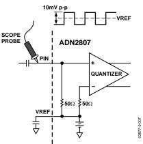
Figure 9. Single-Ended Sensitivity Measurement
