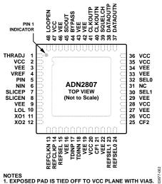
Figure 2. Pin Configuration
