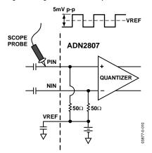
Figure 10. Differential Sensitivity Measurement
