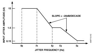
*Figure 12. SONET Jitter Tolerance Mask*
