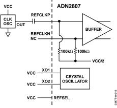
Figure 16. Single-Ended REFCLK Configuration
