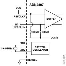
Figure 17. Crystal Oscillator Configuration
