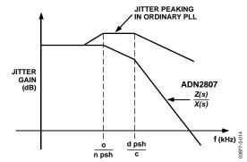
Figure 14. Jitter Response vs. Conventional Phase-Locked Loop
