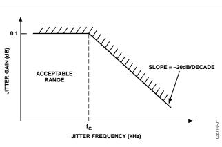
Figure 11. Jitter Transfer Curve
