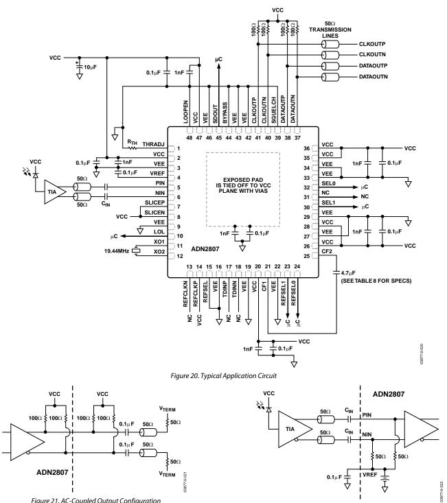
Figure 21. AC-Coupled Output Configuration
