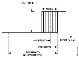
Figure 8. Input Sensitivity and Input Overdrive
