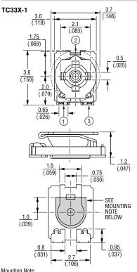
Mounting Note: The gray area can be used to apply cement to hold the unit in place during board processing, if required
