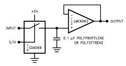
Figure 31. Low-Leakage Sample and Hold
