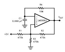
Figure 32. 1 Hz Square Wave Oscillator
