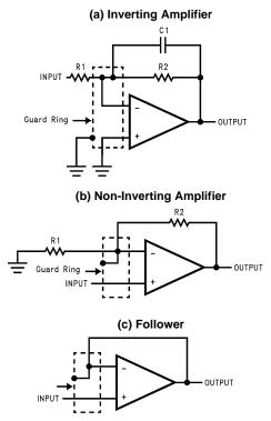
Figure 28. Typical Connections of Guard Rings
