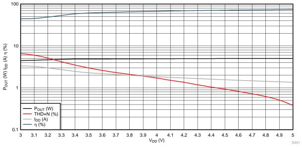
Figure 25. V\_{DD} vs P\_{OUT}, I\_{DD}, and Efficiency With 4- $\Omega$  Load
