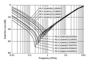
Common Mode Insertion Loss-Frequency Characteristics
