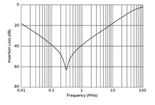
Common Mode Insertion Loss (Typ.)
