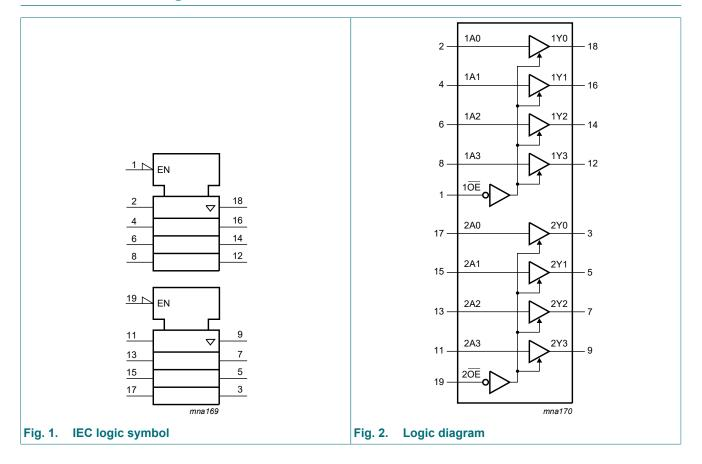
Octal buffer/line driver; 30  $\Omega$  series termination; 5 V tolerant input/output; 3-state
