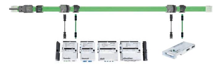
The 7-pole *gesis*®<sub>NRG</sub> BASIC+SELV flat cable 5G2.5+2x1.5 mm<sup>2</sup> supplies energy (3-phase) and the KNX to the area. Consumers/field devices/actuators/module units can then be supplied directly with mains power via 3-pole flat cable adapters with phase selection; the KNX is tapped via a further 2-pole adapter. With the use of Wieland KNX systems, the room automation components are then connected via a *gesis*<sup>®</sup> connecting cable.
