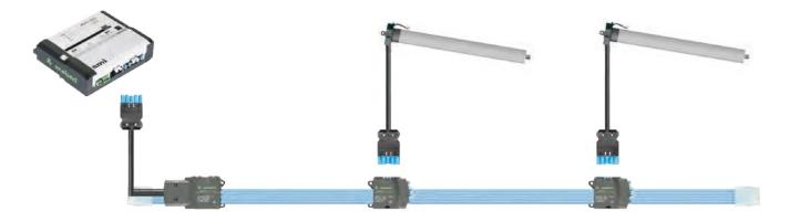
The 5-pole **ge**sis®NRG DIMM flat cable 5G2.5 mm<sup>2</sup> supplies energy (1-phase) and the SMI signal to the area. The drives can then be supplied with mains power and SMI signal directly via 5-pole flat cable adapters. As a rule, **gesis**® connectors are then assembled on the connection cable of the drives. The drives can often be ordered from the manufacturer as already pluggable models (pre-assembled plug).
