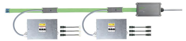
The 5-pole *gesis*®<sub>NRG</sub> flat cable 5G10 mm<sup>2</sup> supplies energy (3-phase, up to 50 A) to the area. Here, *gesis*®<sub>RAN</sub> system distribution units are then connected to pre-assembled connection cables and flat cable adapters. The system distribution units are built to the customer's wishes and contain the necessary protective devices as well as the pluggable outlets needed for the application.
