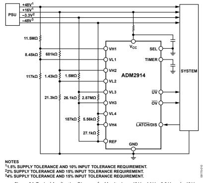
Figure 26. Typical Application Diagram for Monitoring +48 V, +16 V, -3.3 V, and -48 V
