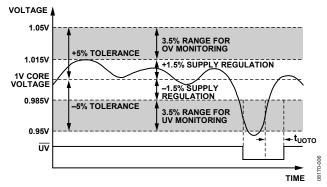
Figure 19. Monitoring Threshold Accuracy Example
