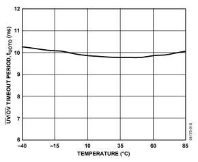
Figure 10. UV/OV Timeout Period vs. Temperature
