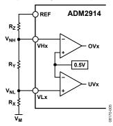
Figure 18. Negative Undervoltage/Overvoltage Monitoring Configuration
