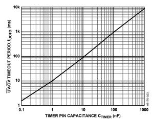
Figure 15. UV/OV Timeout Period vs. Capacitance
