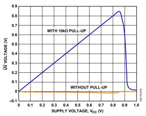
Figure 11.  $\overline{UV}$  Output Voltage vs.  $V_{cc}$
