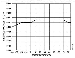
Figure 4. Input Threshold Voltage vs. Temperature
