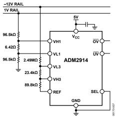
Figure 20. Positive and Negative Supply Monitor Example
