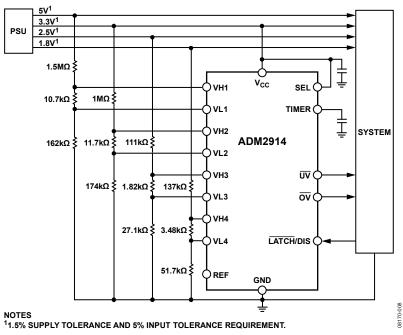
Figure 24. Typical Application Diagram for Monitoring 5 V, 3.3 V, 2.5 V, and 1.8 V
