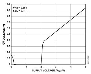
Figure 12. UV Output Voltage vs. Vcc
