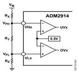
Figure 17. Positive Undervoltage/Overvoltage Monitoring Configuration
