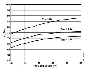
Figure 5. Supply Current vs. Temperature
