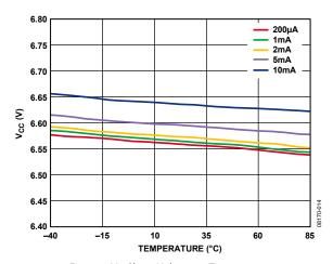
Figure 6.  $V_{CC}$  Shunt Voltage vs. Temperature
