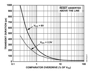
Figure 9. Transient Duration vs. Comparator Overdrive
