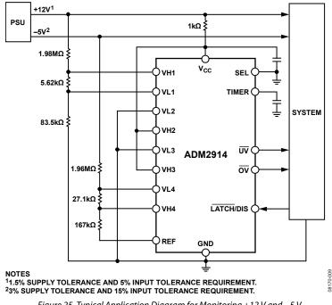
Figure 25. Typical Application Diagram for Monitoring +12 V and -5 V
