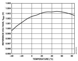
Figure 8. Buffered Reference Voltage vs. Temperature
