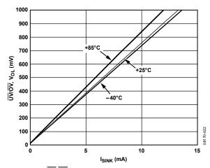
Figure 14.  $\overline{\text{UV}}/\overline{\text{OV}}$  Voltage Output Low vs. Output Sink Current
