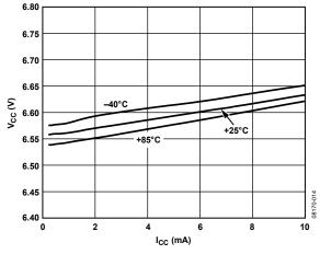
Figure 7. V<sub>CC</sub> Shunt Voltage vs. I<sub>CC</sub>
