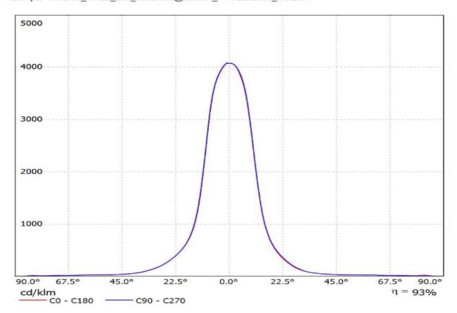
Luminaire: Ledil Oy CS14895\_HB-IP-2X6-RS\_(H35C1)\_SIMULATED Lamps: 1 x LG H35C1
