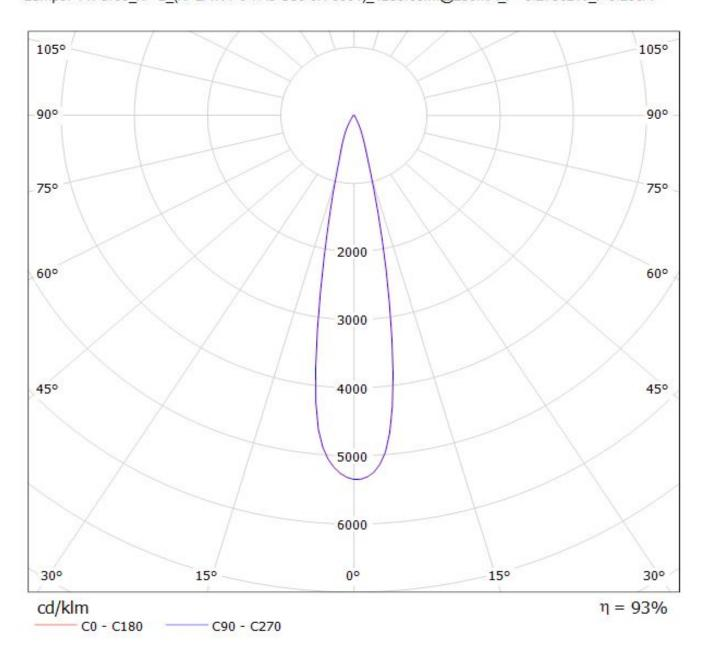
Luminaire: Ledil CS14895\_HB-IP-2X6-RS\_(XP-L2) Lamps: 1 x Cree\_XP-L2\_2x6\_1659.4Im@250mA\_P=8.22525W\_I=0.25A
