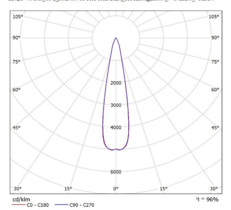
Luminaire: LEDiL Oy CS14895\_HB-IP-2X6-RS Lamps: 1 x Cree\_XP-G2\_1235.27Im@250mA\_P=8.6001W\_I=0.25A
