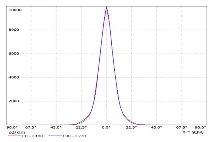
Luminaire: Ledil CS14895\_HB-IP-2X6-RS\_(XR-TX) Lamps: 1 x Luxeon\_XR-TX\_1376.41Im@250mA\_P=8.3920W\_I=0.250A
