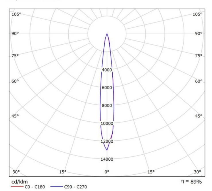
Luminaire: LEDiL Oy CS14895\_HB-IP-2X6-RS\_(Z5M2) Lamps: 1 x Seoul\_Z5M2\_2x6\_(SZ5-M2-W0-00)\_1510.16Im@250mA\_P=8.57039W\_I=0.25A
