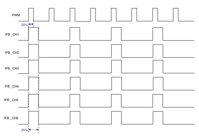
Figure 16. Programmable PWM Dimming Timing Diagram
