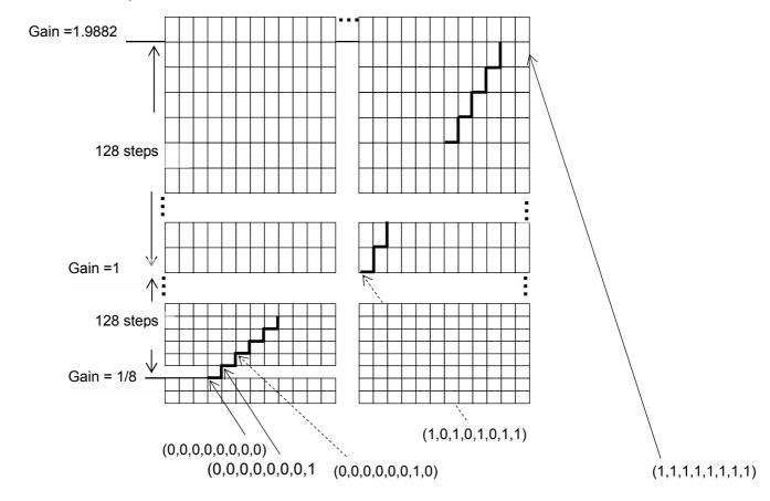
The bit 9 to bit 2 of the configuration register set the gain of output current, i.e., G. As totally 8-bit in number, i.e., ranged from 8'b00000000 to 8'b11111111, these bits allow the user to set the output current gain up to 256 levels. These bits can be further defined inside Configuration Register as follows:
