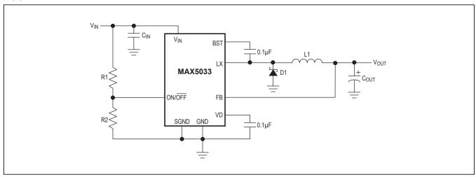
Figure 2. Fixed Output Voltages
