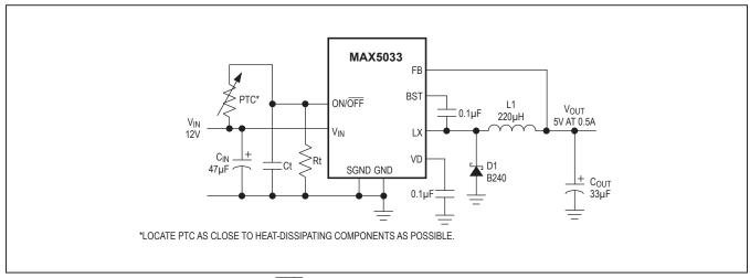
Figure 3. Load Temperature Monitoring with ON/ $\overline{\text{OFF}}$  (Requires Accurate  $V_{\text{IN}}$ )
