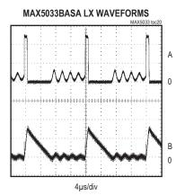
A: SWITCH VOLTAGE, 20V/div, V<sub>IN</sub> = 48V B: INDUCTOR CURRENT, 100mA/div (I<sub>OUT</sub> = 30mA)
