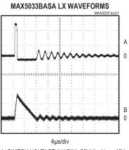
A: SWITCH VOLTAGE (LX PIN), 20V/div, V<sub>IN</sub> = 48V B: INDUCTOR CURRENT, 100mA/div (I<sub>OUT</sub> = 0)
