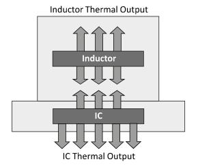
Figure 28 Heat sources in the FS1403
