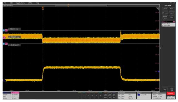
Figure 25 Transient response 0A to 3A (Ch6:I<sub>o</sub>, Ch2: V<sub>out</sub>), peak-peak deviation=79mV
