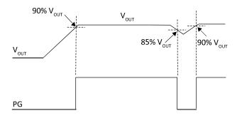
Figure 13 PG signal when PGControl bit=1
