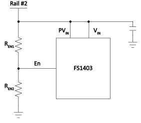
Figure 8 En pin used to monitor other rails for sequencing purposes
