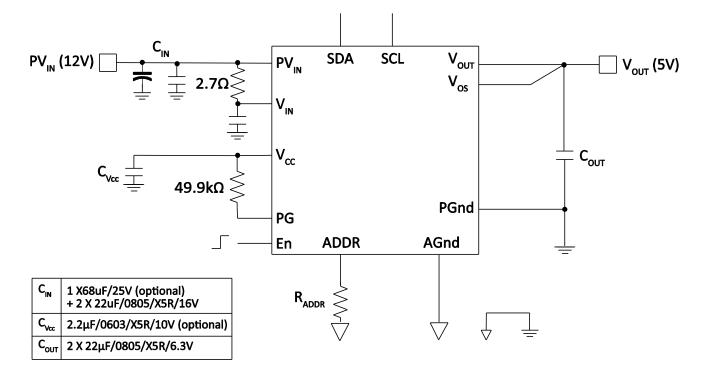
Figure 15 Application circuit for a single supply, PV<sub>IN</sub>=12V, V<sub>OUT</sub>=5V, 3A
