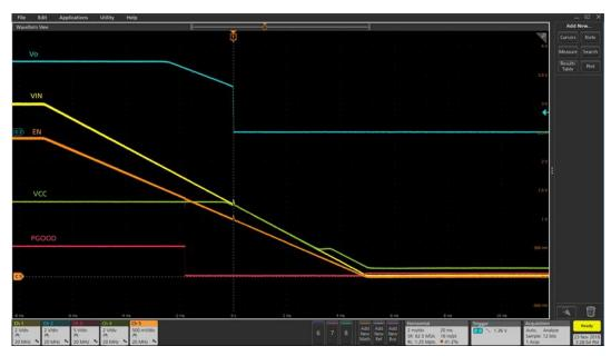
Figure 18 Shutdown with Enable de-assertion at 3A load (Ch1:PV<sub>IN</sub>, Ch2: V<sub>OUT</sub>, Ch3: PGood, Ch4:V<sub>CC</sub>, Ch5: Enable)
