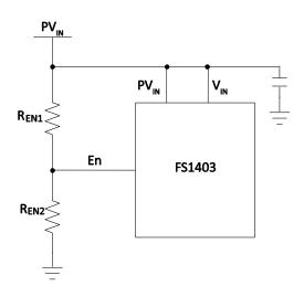
Figure 5 Single supply configuration: internal LDO regulator, adjustable PV<sub>IN</sub>\_UVLO
