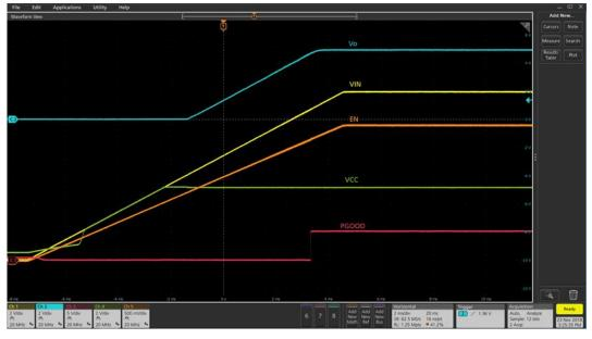
Figure 16 Startup with no load (Ch1:PV<sub>IN</sub>, Ch2: V<sub>OUT</sub>, Ch3: PGood, Ch4:V<sub>cc</sub>, Ch5: Enable)
