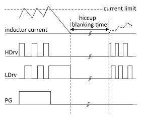
Figure 11 Illustration of OCP in hiccup mode
