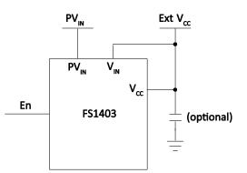
Figure 6 Using an external bias voltage
