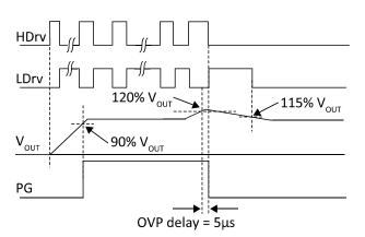
Figure 12 Illustration of latched OVP
