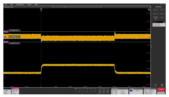
Figure 26 Transient response 1A to 3A (Ch6:I<sub>o</sub>, Ch2: V<sub>OUT</sub>), peak-peak deviation=66mV
