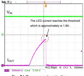
Fig. 74 Over current protection
