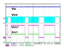
Fig. 73 Thermal protection
