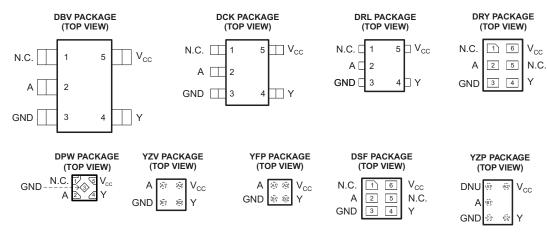
See mechanical drawings for dimensions. N.C. – No internal connection DNU – Do not use
