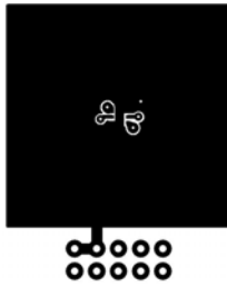
c. 69 °C/W when mounted on a 1 in 2 pad of 2 oz copper
