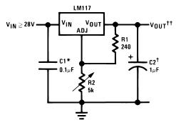
Full output current not available at high input-output voltages
