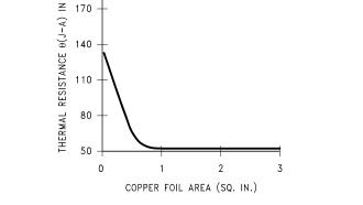
Figure 29.  $\theta_{(J-A)}$  vs Copper (2 ounce) Area for the SOT-223 Package
