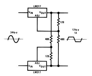
Figure 56. AC Voltage Regulator
