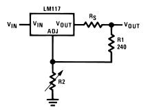
Figure 26. Regulator with Line Resistance in Output Lead
