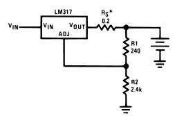
\*R<sub>S</sub>—sets output impedance of charger: Z<sub>OUT</sub> = R<sub>S</sub>  $\left(1 + \frac{R_2}{R_1}\right)$
