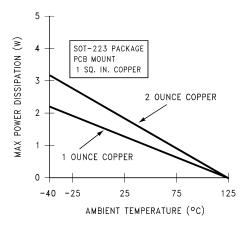
Figure 30. Maximum Power Dissipation vs T<sub>AMB</sub> for the SOT-223 Package
