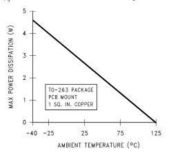
Figure 32. Maximum Power Dissipation vs T<sub>AMB</sub> for the TO-263 Package
