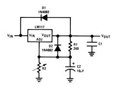
$$\begin{split} & V_{OUT} = 1.25V\left(1+\frac{R2}{R1}\right) + I_{ADJ}R2 \\ & D1 \text{ protects against C1} \\ & D2 \text{ protects against C2} \end{split}$$
