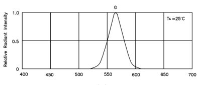
wavelength  $\lambda$  (nm) RELATIVE INTENSITY Vs. WAVELENGTH
