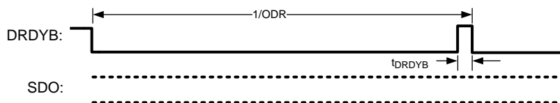
Figure 62. DRDYB Behavior for an ADC_DOUT not Read
