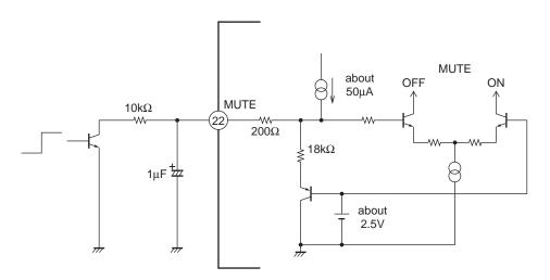
Fig2 Mute equivalent circuit
