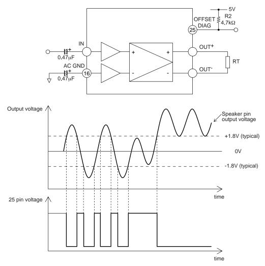
Fig3 Self-diagnosis Function Diagram
