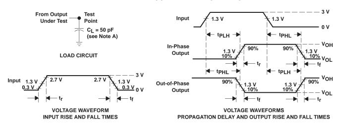
NOTES: A.  $C_L$  includes probe and test-fixture capacitance.
