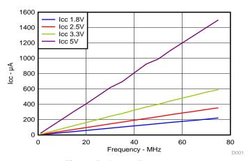
Figure 5. I<sub>CC</sub> vs Frequency
