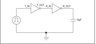
Figure 1. Driver Test Circuit
