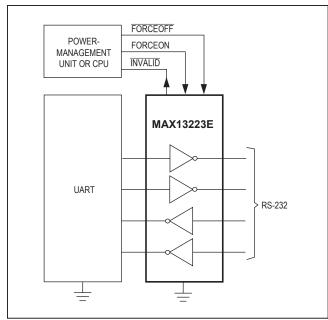
Figure 5. Interface Under Control of PMU
