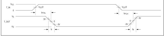
Figure 3. Driver Propagation Delay
