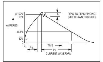
Figure 8b. Human Body Current Waveform
