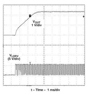
Figure 8. Prebiased Startup Timing
