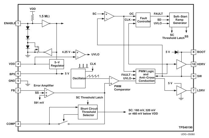
Internally fixed switching frequency and soft-start time reduce external component count, simplifying design and layout, as well as reducing footprint and cost. The 3 mm  $\times$  3 mm package size also contributes to a reduced overall converter footprint.
