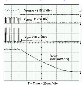
Figure 6. Shutdown Using ENABLE Pin
