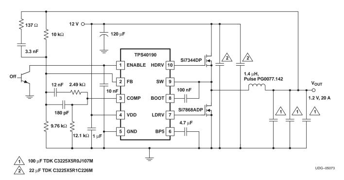
Figure 10. 12-V to 1.2-V at 20 A
