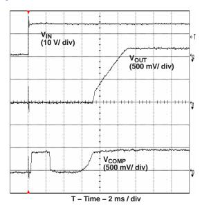
Figure 7. TPS40190 Startup Timing
