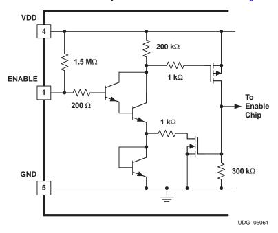
Figure 4. TPS40190 ENABLE Pin Internal Circuitry
