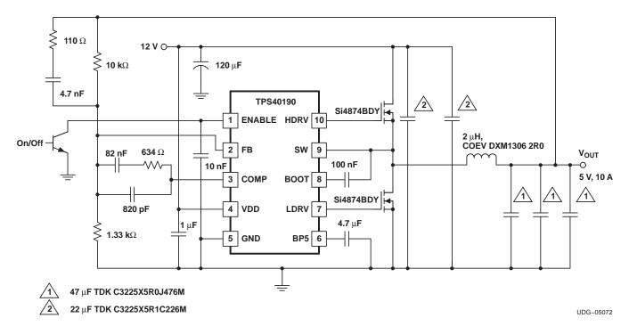
Figure 9. 12-V to 5-V at 10 A
