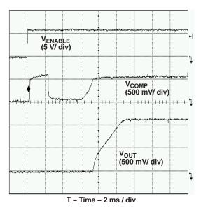
Figure 5. Startup Using ENABLE Pin
