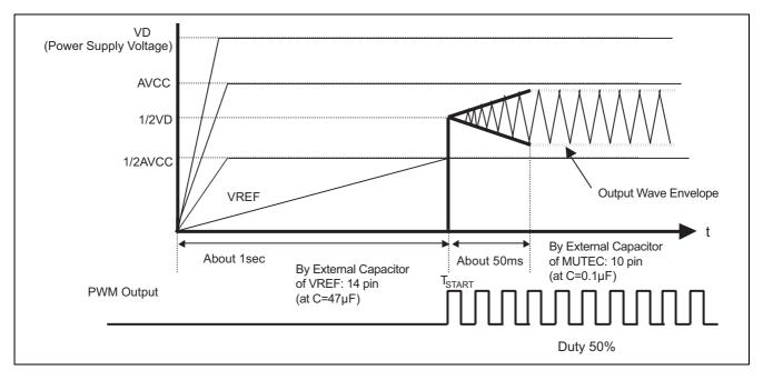
$T_{\text{START}}$  means the time by reached VREF to 1/2Avcc and determined automatically by the value of capacitor  $C_{\text{REF}}$  connected to external parts according to the following formula.
