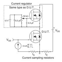
Fig. 13b - Gate Charge Test
