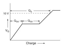
Fig. 13a - Basic Gate Charge Waveform
