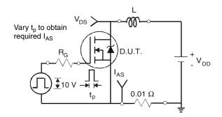
Fig. 12a - Unclamped Inductive Test Circuit
