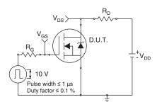
Fig. 10a - Switching Time Test Circuit
