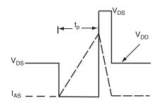
Fig. 12b - Unclamped Inductive Waveforms
