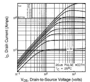
Fig. 1 Typical Output Characteristics, T<sub>C</sub> = 25 °C
