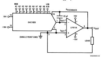
$$V_{OUT} = -V_{REF} \left( \frac{A1}{2} + \frac{A2}{4} + \frac{A3}{8} + \cdots \frac{A10}{1024} \right)$$
