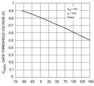
T<sub>ch</sub>, CHANNEL TEMPERATURE (°C) Fig. 3 Gate Threshold Voltage vs. Channel Temperature
