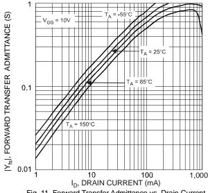
Fig. 11 Forward Transfer Admittance vs. Drain Current
