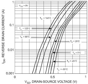
Fig. 10 Reverse Drain Current vs. Source-Drain Voltage
