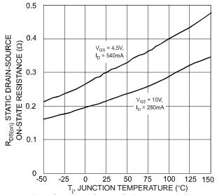
Fig. 8 Static Drain-Source, On-Resistance vs. Temperature
