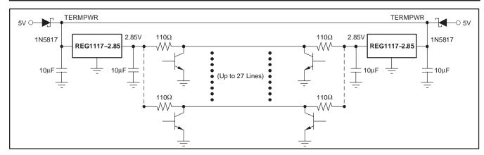
Figure 7. SCSI Active Termination Configuration
