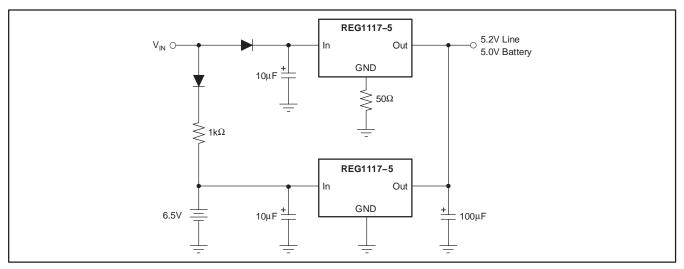
Figure 10. Battery Backed-Up Regulated Supply
