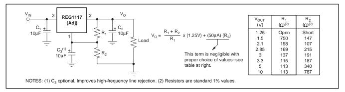
Figure 2. Adjustable-Voltage Model—Basic Connections
