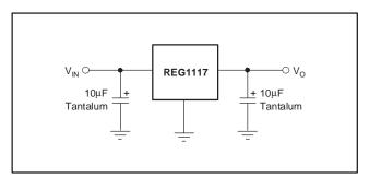
Figure 1. Fixed-Voltage Model—Basic Connections
