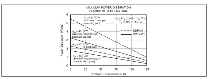
Figure 6. Maximum Power Dissipation versus Ambient Temperature
