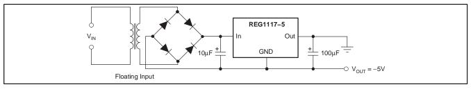
Figure 11. Low Dropout Negative Supply
