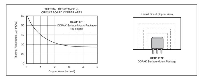
Figure 4. DDPAK Thermal Resistance versus Circuit Board Copper Area
