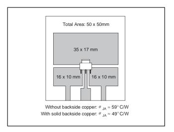
Figure 5. SOT-223 Circuit Board Layout Example
