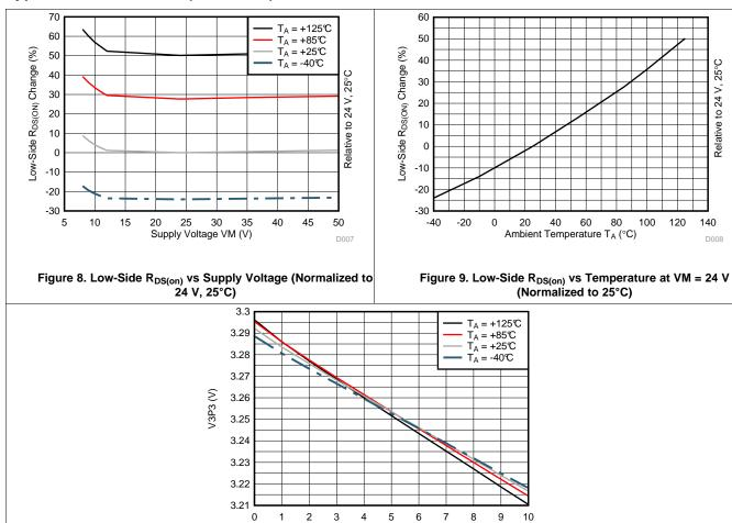
Figure 10. V3P3 Regulator vs Load at VM = 24 V
