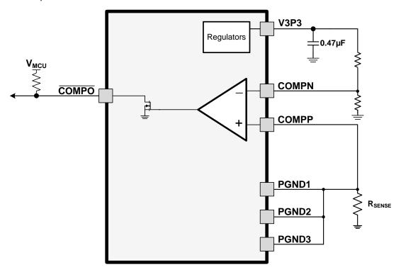
Figure 12. Comparator As Current Monitor
