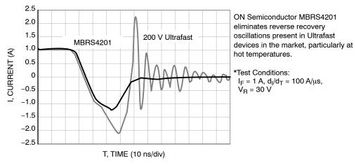
Figure 8. Reverse Recovery Time\* (t<sub>RR</sub>) at 125°C
