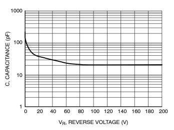
Figure 5. Typical Capacitance
