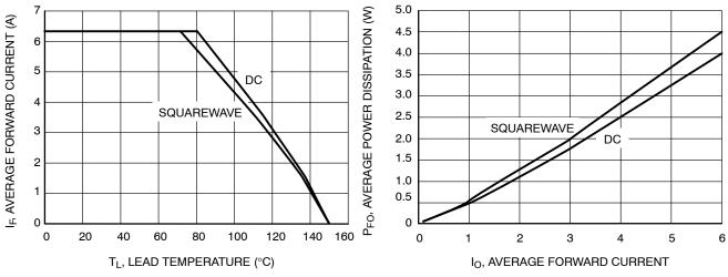
Figure 6. Derating Curve
