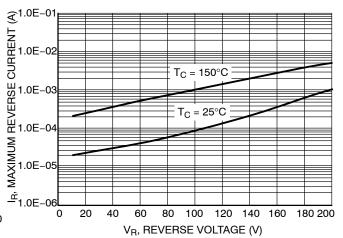
**Figure 3. Typical Reverse Current**
