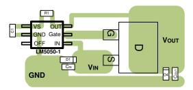
Figure 34. Typical Layout Example With D2PAK N-MOSFET
