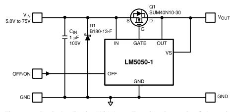
Figure 30. Basic Application With Input Transient Protection Schematic
