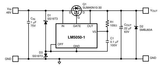
Figure 31. 48-V Application With Reverse Input Voltage ( $V_{IN} = -48 \text{ V}$ ) Protection Schematic
