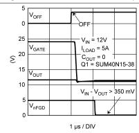
Figure 17. C<sub>GATE</sub> Charge and Discharge vs OFF Pin
