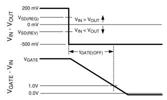
Figure 1. Gate OFF Timing for Forward to Reverse Transition
