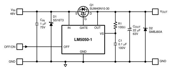
Figure 24. Typical Application With Input and Output Transient Protection Schematic
