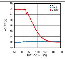
Figure 11. Forward  $C_{GATE}$  Charge Time,  $C_{GATE}$  = 47 nF
