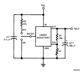
$V_{OUT} = Reference Voltage \times \frac{R1 + R2}{R1}$
