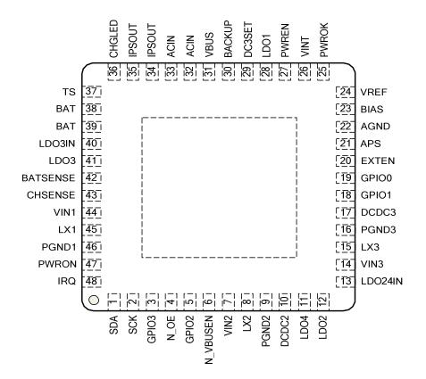
Figure 2. AXP202 Pin Configuration
