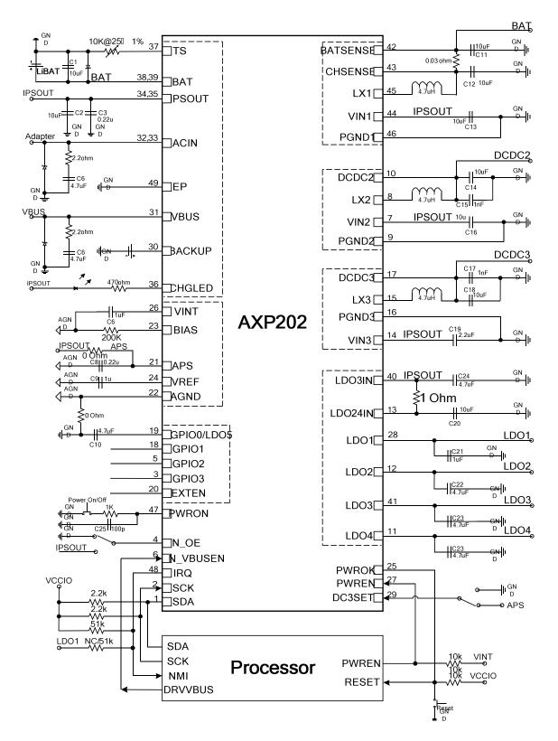
Figure 1. Typical Application Circuit
