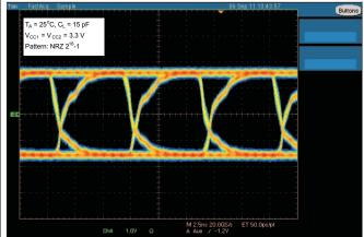
Figure 20. Typical Eye Diagram at 150 Mbps, 3.3-V Operation
