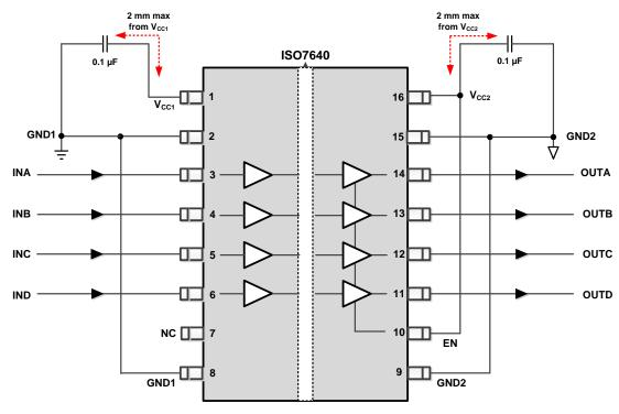
Figure 17. Typical ISO7640FM Circuit Hookup
