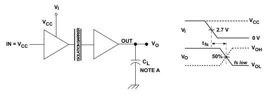
A.  $C_L = 15 \text{ pF}$  and includes instrumentation and fixture capacitance within  $\pm 20\%$ .
