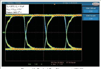
Figure 19. Typical Eye Diagram at 150 Mbps, 5-V Operation
