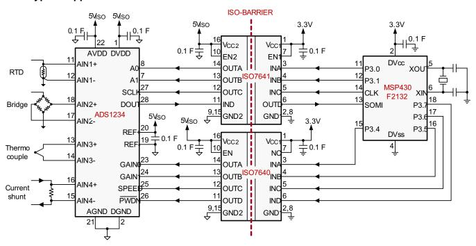
Figure 16. Isolated Data Acquisition System for Process Control
