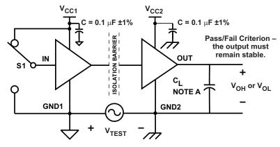
A.  $C_L = 15 \text{ pF}$  and includes instrumentation and fixture capacitance within  $\pm 20\%$ .
