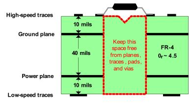
Figure 21. Recommended Layer Stack
