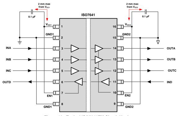
Figure 18. Typical ISO7641FM Circuit Hookup
