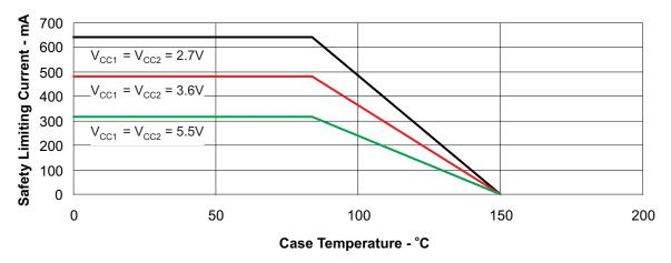
Figure 14. DW-16 θ<sub>IC</sub> Thermal Derating Curve per DIN V VDE V 0884-10
