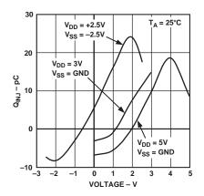
TPC 16. Charge Injection vs. Source Voltage
