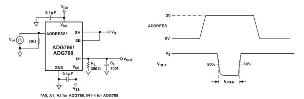
Test Circuit 6. Break-Before-Make Delay, t<sub>OPEN</sub>
