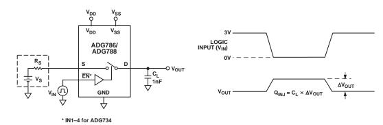
Test Circuit 7. Charge Injection
