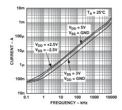
TPC 13. Input Current,  $I_{DD}$  vs. Switching Frequency
