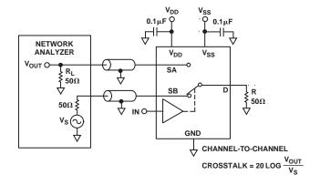
Test Circuit 9. Channel-to-Channel Crosstalk
