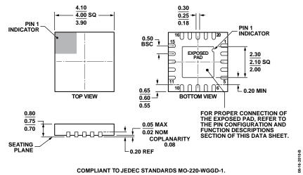
Figure 1. 20-Lead Lead Frame Chip Scale Package [LFCSP] 4 mm × 4 mm Body and 0.75 mm Package Height (CP-20-6) Dimensions shown in millimeters
