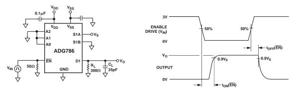
Test Circuit 5. Enable Delay,  $t_{ON}$  ( $\overline{EN}$ ),  $t_{OFF}$  ( $\overline{EN}$ )
