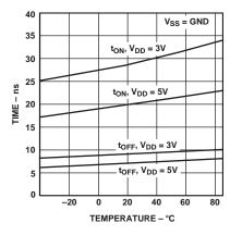
TPC 11.  $t_{ON}/t_{OFF}$  Times vs. Temperature
