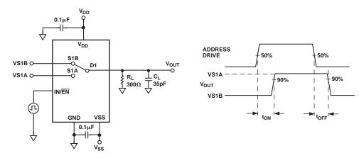
Test Circuit 4. Switching Times, t<sub>ON</sub>, t<sub>OFF</sub>
