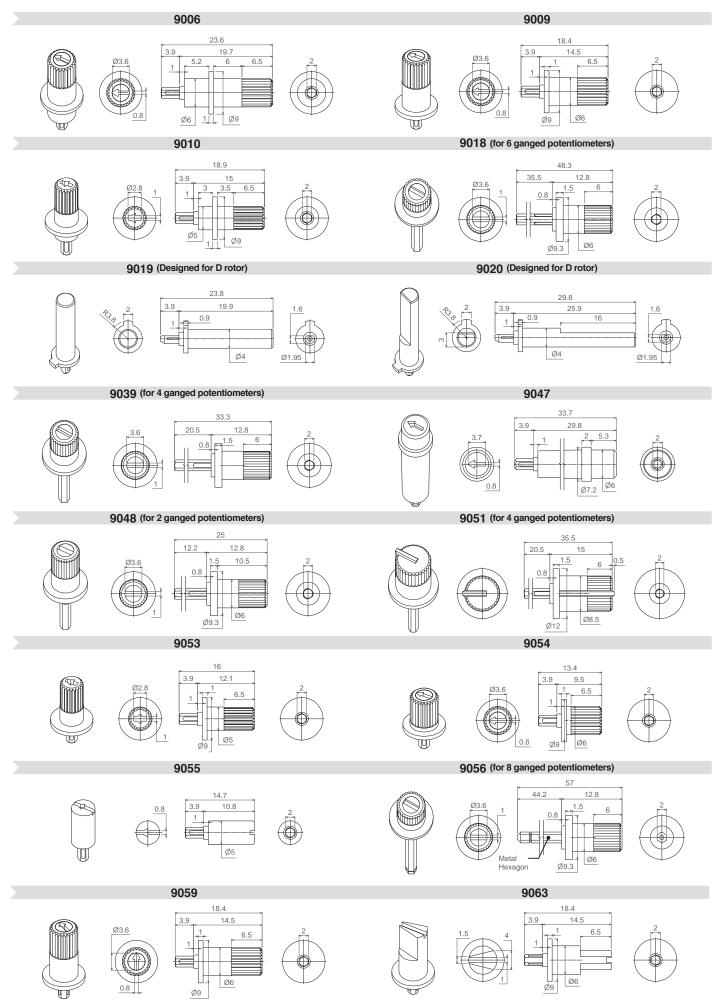
The arrow is in line with the wiper when potentiometer has rotor J (with M rotor, there is a  $30^{\circ}$  difference).
