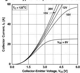
Figure 4. Transfer Characteristics
