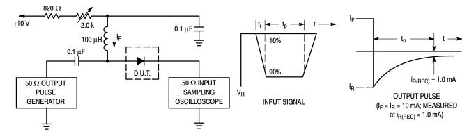
Notes: 1. A 2.0  $k\Omega$  variable resistor adjusted for a Forward Current (I\_F) of 10 mA.
