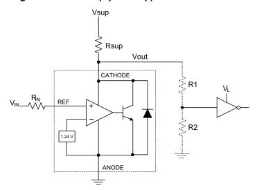
Figure 26. Comparator Application Schematic
