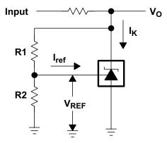
Figure 23. Test Circuit for  $V_{KA} > V_{REF}$ ,  $V_O = V_{KA} = V_{REF} \times (1 + R1/R2) + I_{ref} \times R1$
