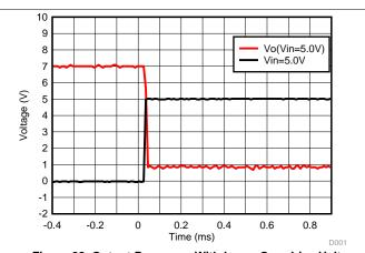
Figure 28. Output Response With Large Overdrive Voltage
