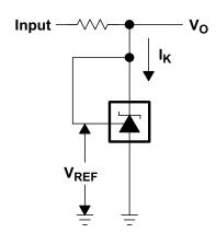
Figure 22. Test Circuit for  $V_{KA} = V_{REF}$ ,  $V_O = V_{KA} = V_{REF}$
