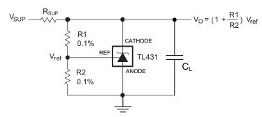
Figure 29. Shunt Regulator Schematic
