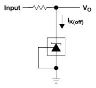
Figure 24. Test Circuit for I<sub>K(off)</sub>
