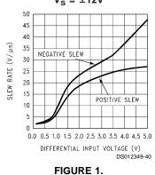
This effect is most noticeable at higher supply voltages and lower gains where incoming signals are likely to be large.
