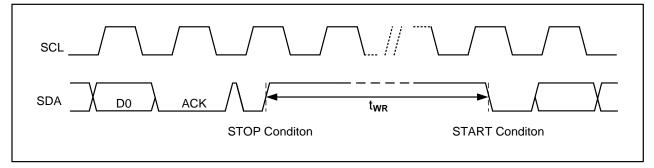
Note: [1] The write cycle time twe is the time from a valid stop condition of a write sequence to the end of the internal clear/write cycle.
